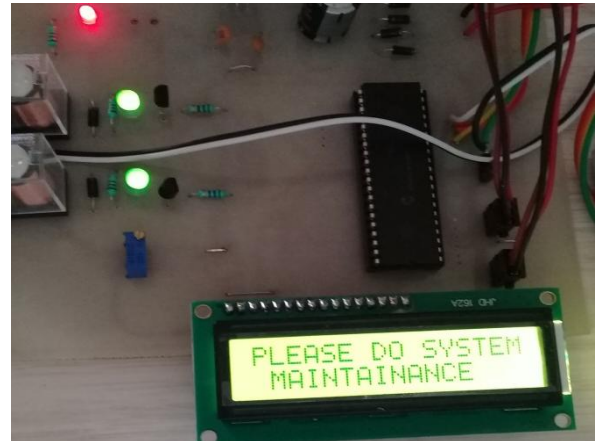
Fig.20: Machine is OFF and allows for system maintenance
