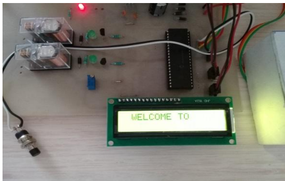
Fig.6: LCD shows message 'WELCOME TO'
